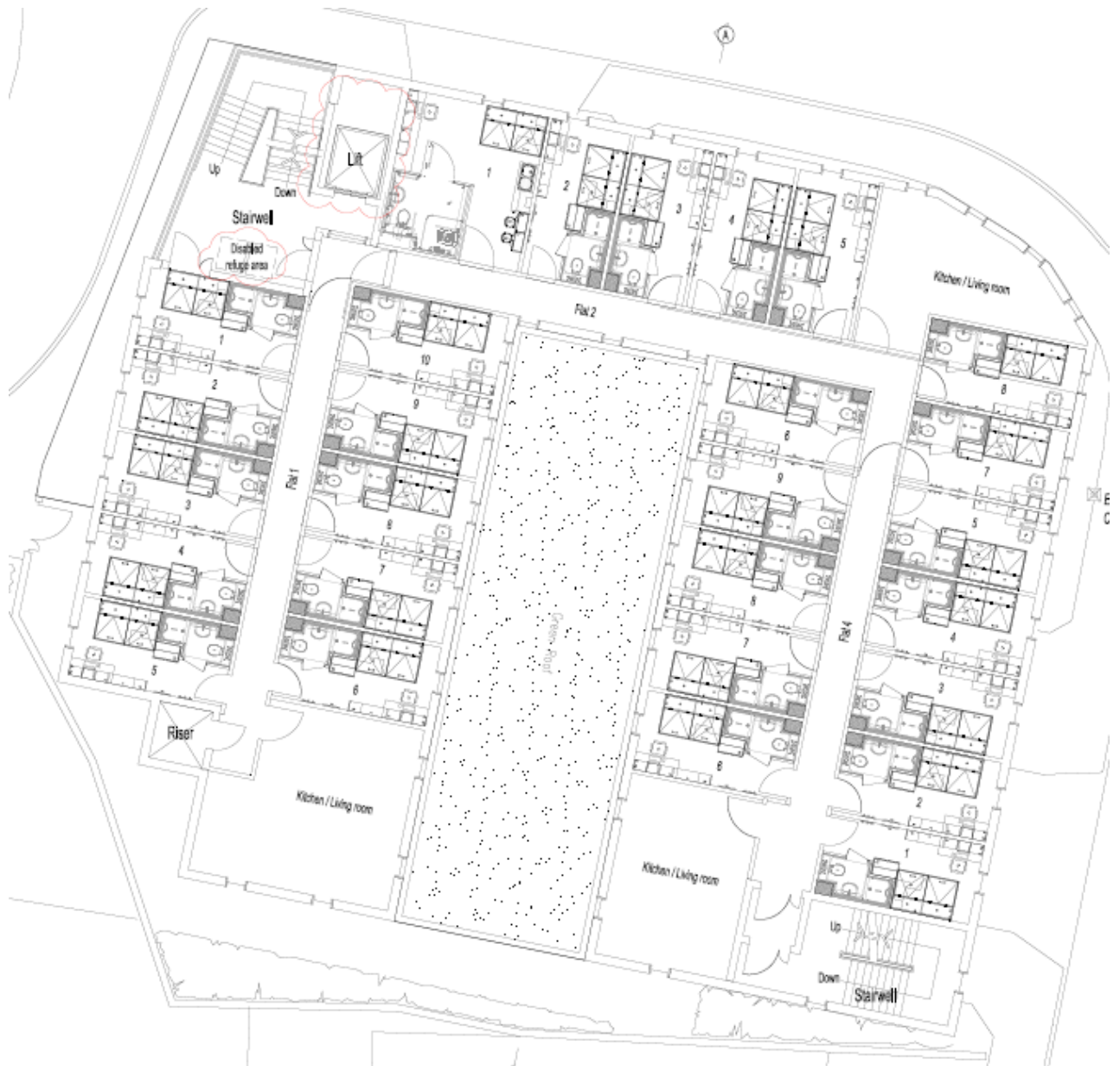
Indicative First Floor Plan (Effectively the same for Floors 2 and 3)
