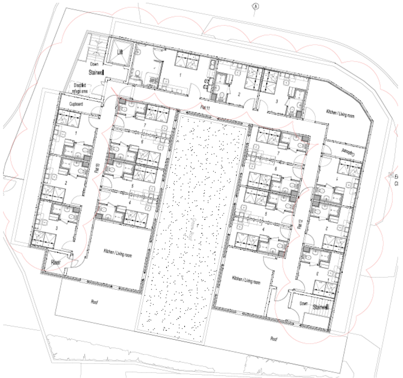
Indicative Fourth Floor Plan (Inset to Mirror Height Plan)
